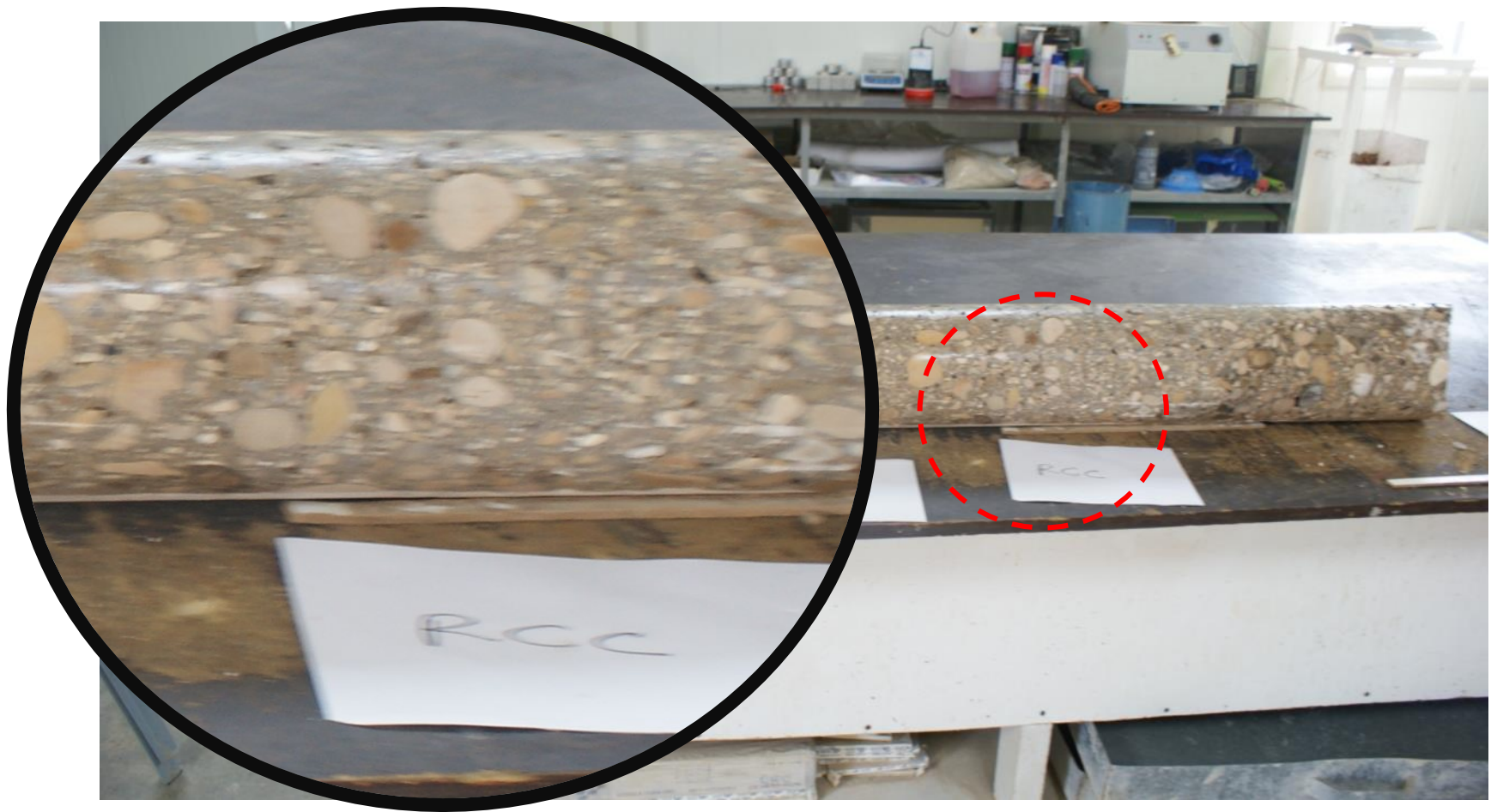
RCC extracted cores' inspection and preparation for testing in Site Laboratory
